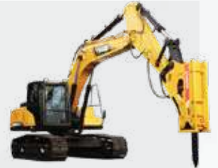
Excavator with Rock Breaker
